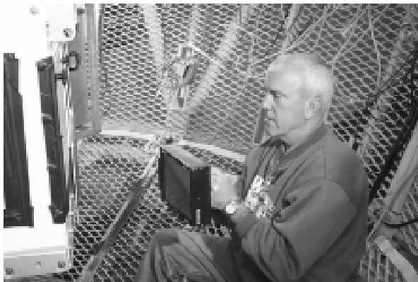
Frank Freeman is at the Cassegrain focus of the telescope preparing the RGO spectrograph for observing, here seen changing the diffraction grating.
