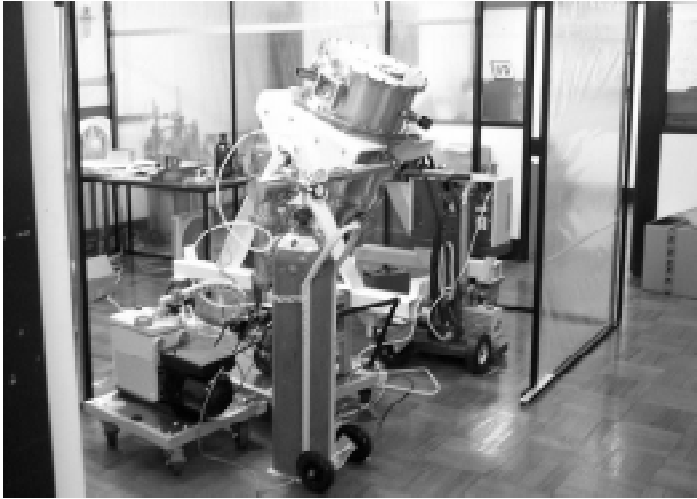
IRIS 2 shells undergoing first pump down and leak test. The fore dewar is clearly visible.
