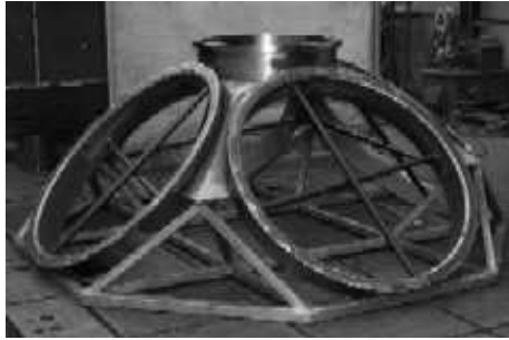
OzPoz Exchanger - revolver structure ready to machine
