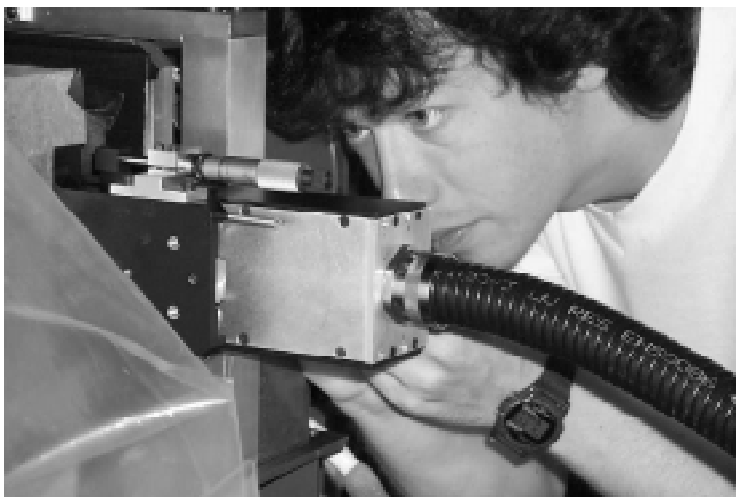
AAO instrument scientist David Lee carefully adjusting the output slit of the SPIRAL instrument during commissioning.
