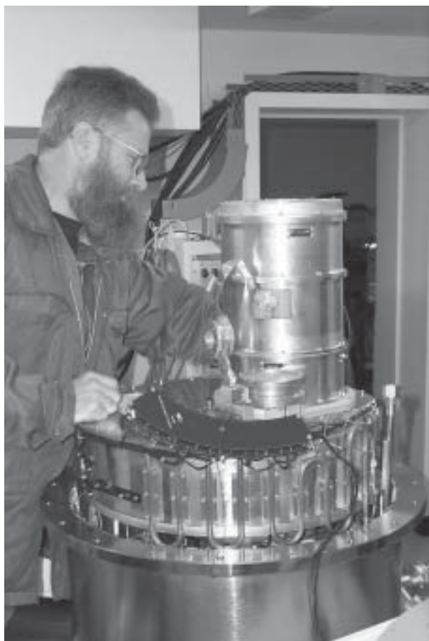
Michael Kanonczuk of the mechanical section at the telescopes is shown dismantling IRIS2 in preparation for adjusting the grisms
