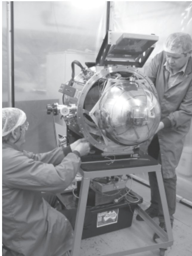
Denis Whittard (left) and Vlad Churilov installing the liquid nitrogen can for AAOmega's blue camera, (photo: Jurek Brzeski)
