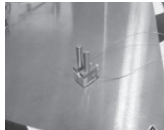
Starbugs - microrobotic actuators - provide a precise, fast and flexible method of positioning multiple payloads in the focal plane of telescopes, to pick out small objects or regions of interest. Shown here are three prototype actuators developed at the AAO. Photos Jurek Brzeski
