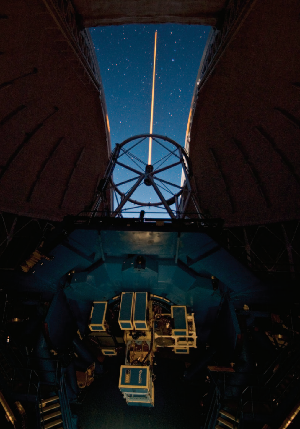
Figure 1. Gemini North's laser propagating up into the sky above Mauna Kea in Hawaii. The blue-and-white boxes mounted behind the primary mirror in the lower half of this image contain the instruments that make use of the artificial star created by the laser to compensate for the blurring effect of the Earth's atmosphere. Image courtesy of Gemini Observatory/AURA.
