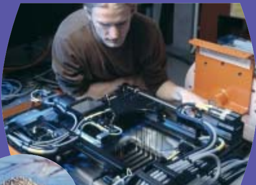
FMOS-Echidna — a radical new fibre-positioner being built for Japan's Subaru Telescope. Its 400 fibres will be individually positioned by piezoelectric drivers. Photograph: David James
