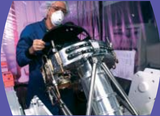
IRIS2 — a widefield infrared camera and spectrograph. In 2002 it won Engineers Australia's JJC Bradfield Award for outstanding engineering achievement. Photograph: David Smyth
