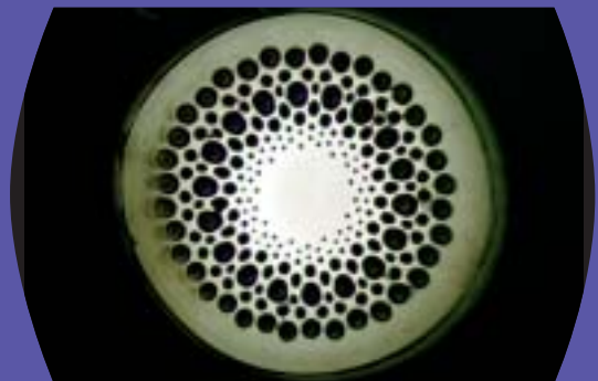
Customised optical fibres — being developed with commercial partners. Image: OFTC, University of Sydney.
