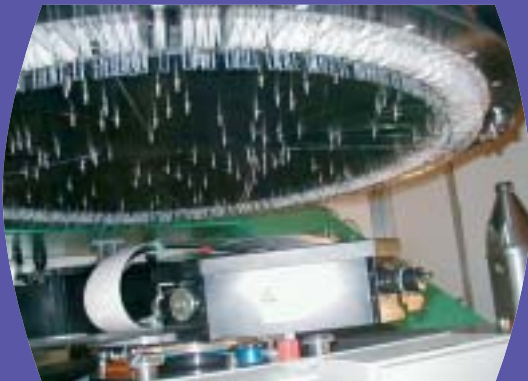
Oz-Poz — a multi-fibre positioner for the European Southern Observatory's Very Large Telescope in Chile.
